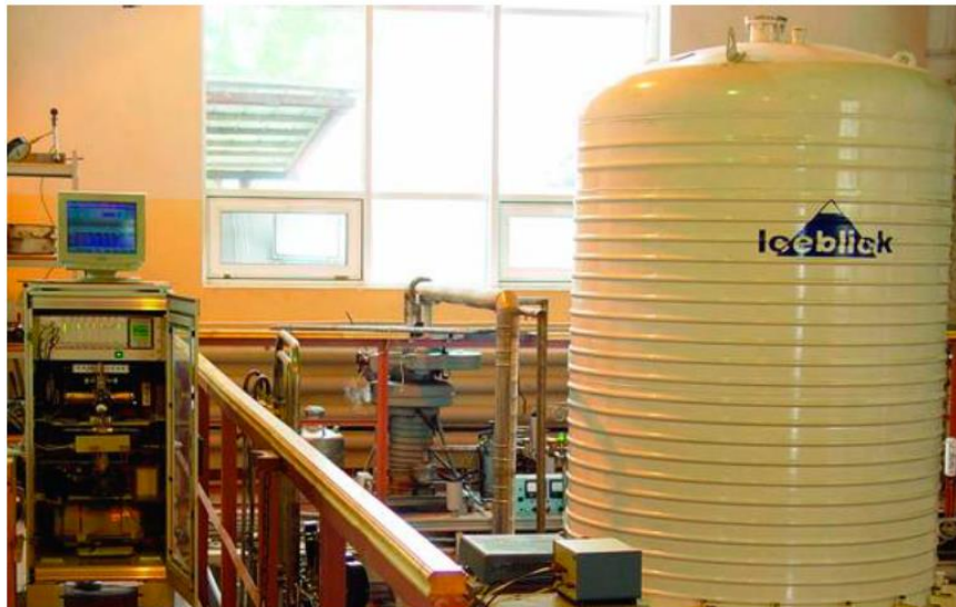
GAOS MS-20-9 mass spectrometer. Determination of the micro impurities, high purity neon production (99,9999 %), «IceBlick», Odessa
