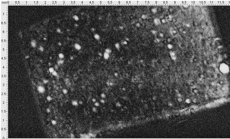
Acoustic image (C-scan) of interior structure in the middle of the specimen thickness.
