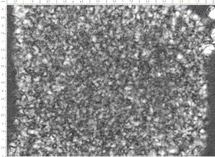
Acoustic image (C-scan) of interior structure in the middle of the specimen depth.
