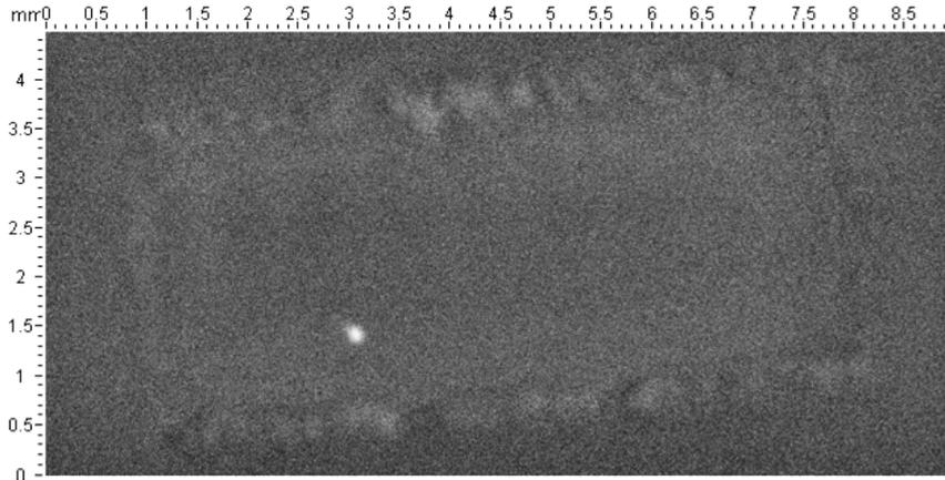
Acoustic image (C-scan) of interior structure in the middle of the specimen thickness.
