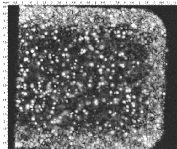
Acoustic image (C-scan) of interior structure in the middle of the specimen thickness.
