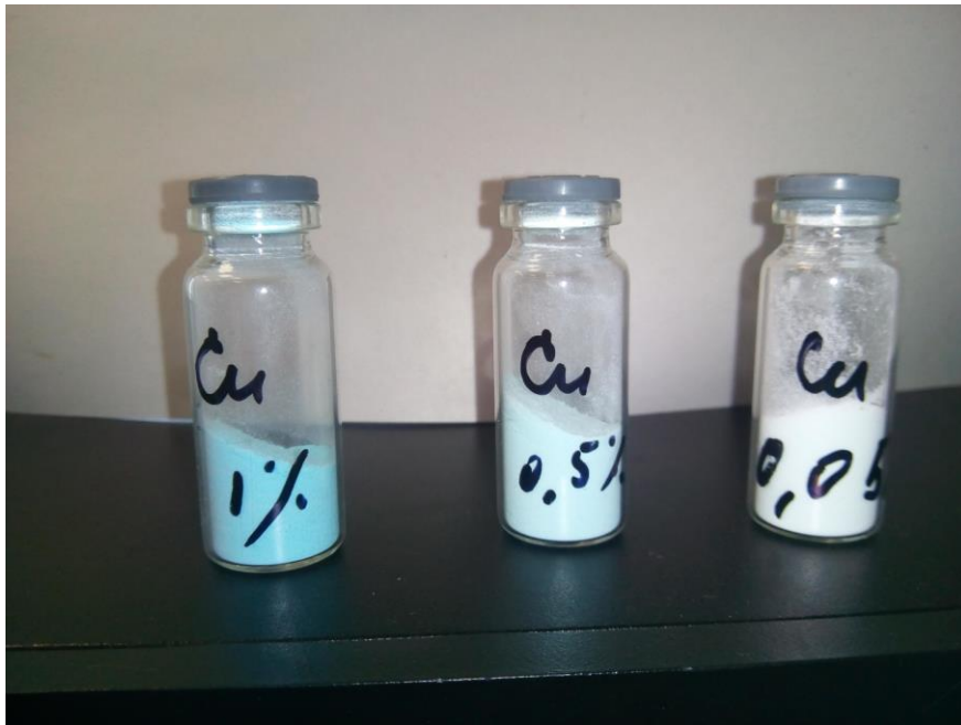
Fig. 2. Mixtures of boric acid with copper oxide
