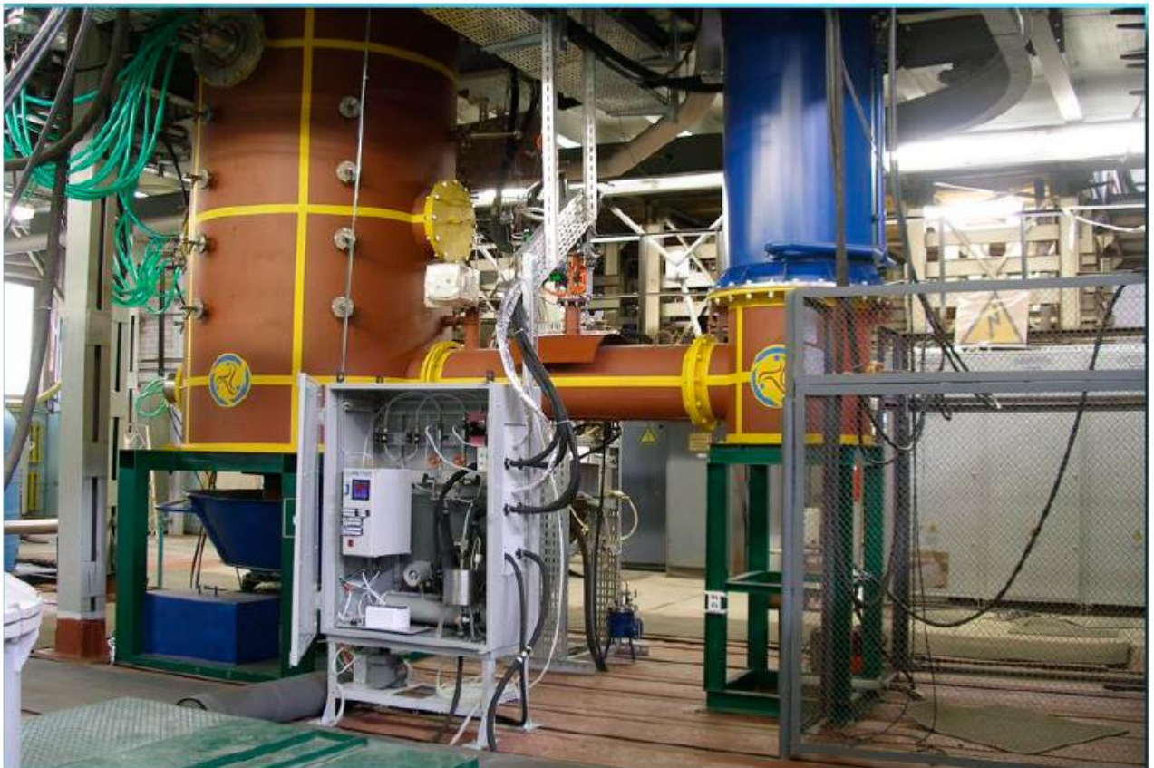
Experimental installation of plasma gasification of solid waste at the Institute of Electrophysics and Power Engineering, St. Petersburg. In the foreground is a system for sampling and processing samples of a gas-analytical complex based on GAOS MS-20-1 mass spectrometer.
