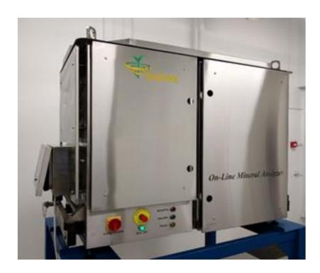
Ostec-Instruments offers the industrial chemistry analyzer **LIOS OnLine** intended for quick and safe check of processes by means of continuous on-stream analysis of product's chemical composition directly on conveyor belts or in pipelines for suspensions/liquids if such analyses are made on a real-time basis exclusive of sampling, delay in laboratory analysis and any types of hazardous radiation.
