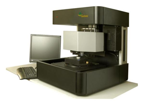
XROS MF30 – laboratory x-ray microscope-microprobe for studies of the objects by the methods of the optical microscopy, radiography, local element XRF microanalysis with possibility of the element mapping. Using a microscope, a sample of up to 400 mm in size along the Y axis and of unlimited size along the X axis (max. scan area 150×150 mm; in the case of a larger area, the scanned areas can be stitched) and up to 105 mm high can be performed.
